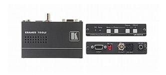
The VP-501N is a scan converter for computer graphics and HDTV component video signals. It converts the input up to UXGA (1600x1200) and HDTV (1080p) to composite and s-Video (Y/C) signals simultaneously in either PAL or NTSC formats.
